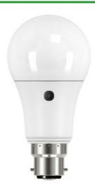
The LED Photocell GLS is the ideal lamp to reduce the amount of wasted energy while increasing security at any premises. With automatic dusk till dawn switching, this lamp is the lamp of choice for applications such as porches, hallways and suitable IP rated outdoor fixtures.
