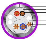
LSZH SHEATH TINNED COPPER BRAID AL-PET SCREEN PE INSULATION STRANDED TINNED COPPER CONDUCTOR COTTON ROPE TINNED COPPER DRAIN WIRE
