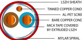
TINNED COPPER CONDUCTOR – AL-PET SCREEN BARE COPPER CONDUCTOR
